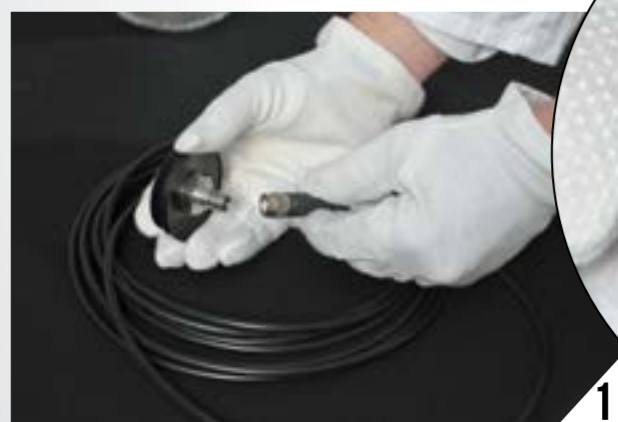
1 Connect de GPS antenna to RSN279 cable or TNC/TNC adaptor.
