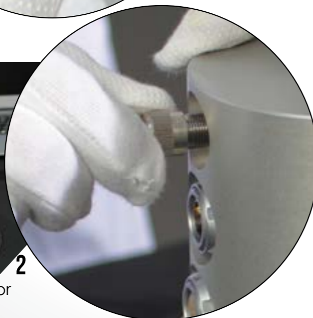
1 Connect de GPS antenna to RSN279 cable or TNC/TNC adaptor.
